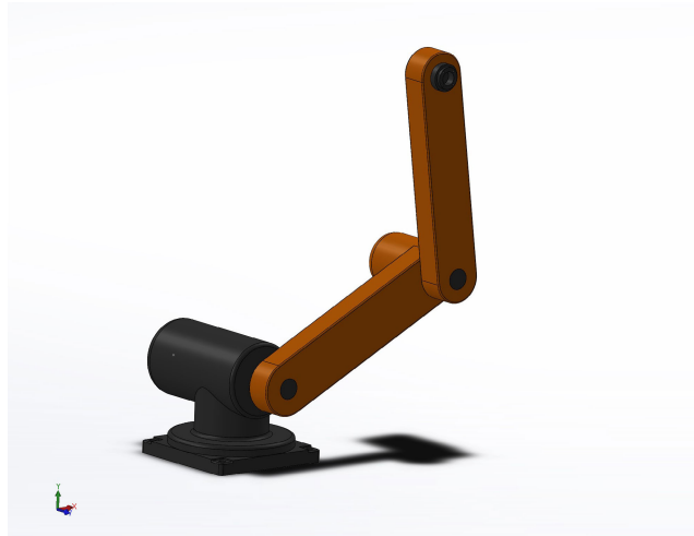
FIGURE 2. 2-DOF robotic mechanical model in SOLIDWORKS.
