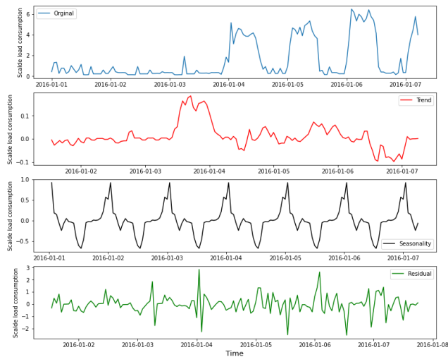
FIGURE 2. Original load series data and its decomposition. As this data is an hourly data, it has every 24 hours seasonality.
