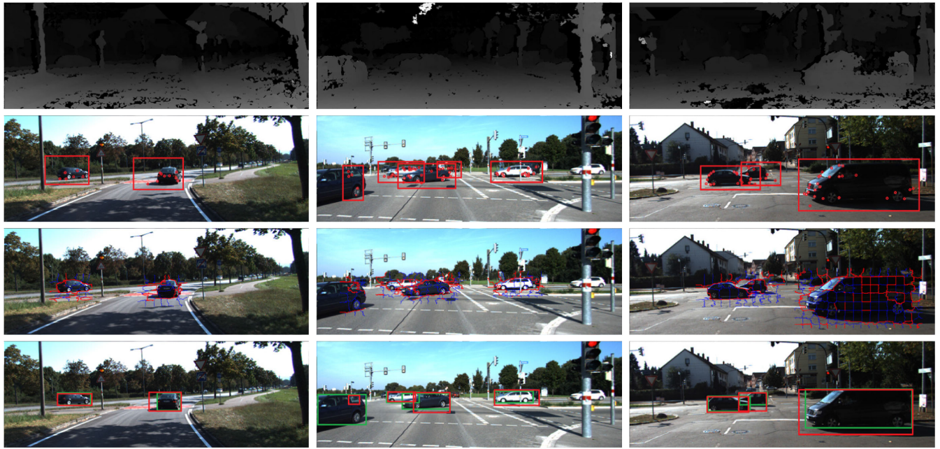
FIGURE 8. Examples of dynamic area detection on KITTI benchmark. First row, disparity images obtained by SGBM; second row, dynamic regions of interest; third row, results of SLIC and boundary marking; fourth row, dynamic areas (red rectangles) and ground truths (green rectangles).
