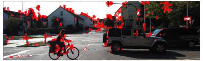
(a) FAST extractor in OpenCV
