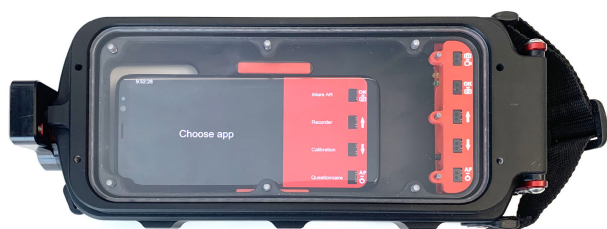
(b) The marker-based AR system runs on a Samsung S8 sealed in Diveshot, a waterproof housing from Easydive. Divers operate the lower four buttons that correspond to the four buttons of the application, and the fifth, top-most button is used by the supervisor to access and change the application settings.
