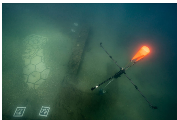
FIGURE 2. Underwater site after the setup of both the systems. Notice two pairs of markers representing two anchors located in corners of the room in the left part of the image, and the base of the acoustic localization system in the right part of the image.
