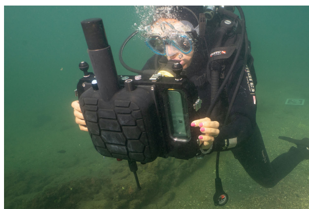
FIGURE 6. The new underwater case coupled with the acoustic localization system.
