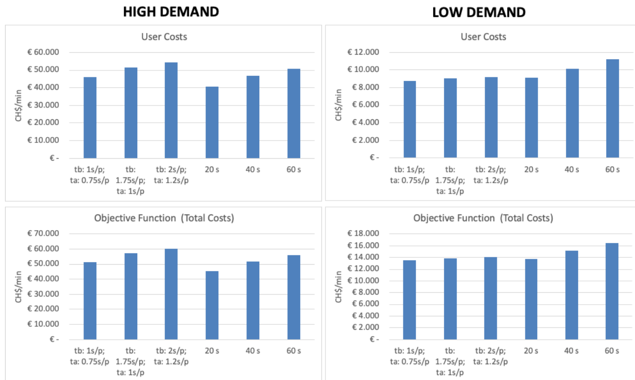
FIGURE 10. Comparative analysis of user costs and objective function for different dwell time values at high demand (left) and low demand (right).
