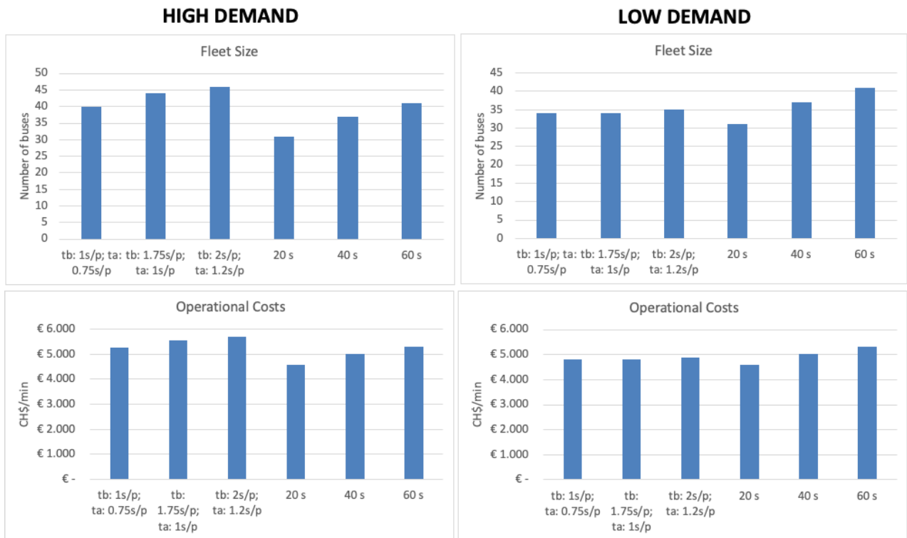
FIGURE 9. Comparative analysis of operational costs and fleet sizes for different dwell times at high (left) and low (right) demand levels.
