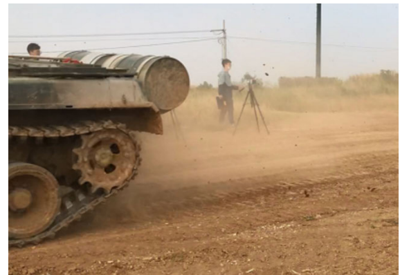
FIGURE 11. Measurement process of the dust mass concentration.
