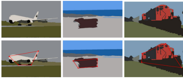
FIGURE 7. Geometrical shape features extraction using Euclidian distance.
