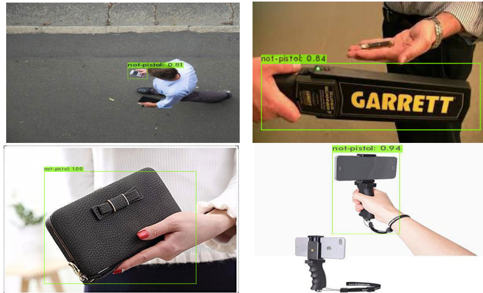
FIGURE 18. Detection Results- Top left to bottom right (a-d): (a) Cell phone (b) Metal detector(c) Wallet (d) Selfie stick.
