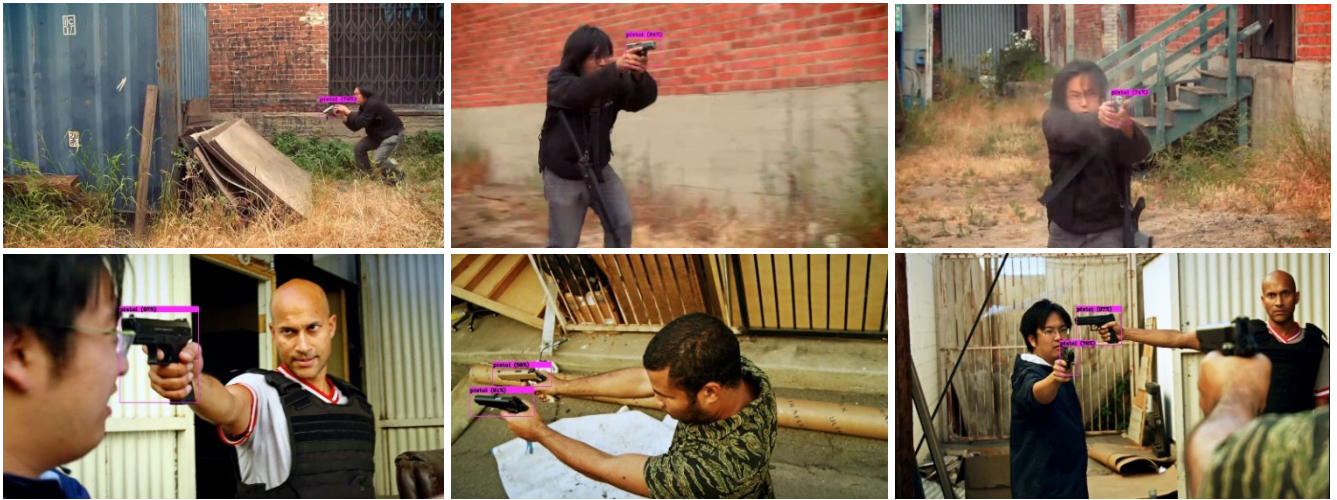
FIGURE 16. Detection Results-Top left to bottom right (a-f) - video 1 inference (a-c), video 2 inference (d-f): (a) Small object-side view tilted, (b) Small object with side view (c) Small object front view (d) side view (e) Top view double object (f) Small object with front and side view.
