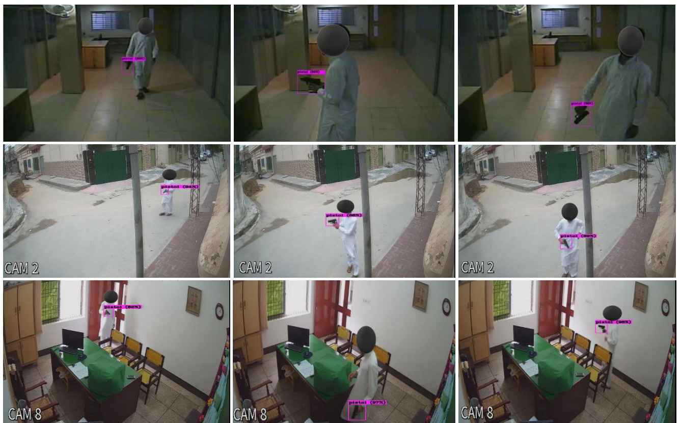
FIGURE 17. Detection Results-Top left to bottom right (a-i)-cctv stream1(a-c),cctv stream2(d-f), cctv stream3(g-i): (a) Small object in Low resolution (b) Tilted Object (c) Low Resolution vertical object, (d) Day light side view with slightly tilted (e) Day light side view (f) Day light side view flipped (g) Small object medium resolution (h) vertical view (i) side view.
