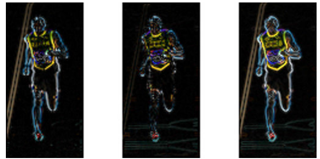
FIGURE 3. Gradient magnitude map (left: x direction; middle: y direction; right: gradient magnitude).
