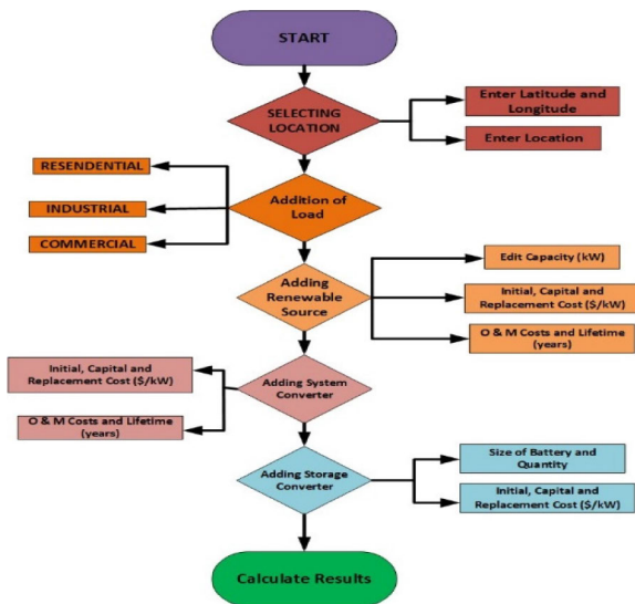
FIGURE 4. The methodology used in HOMER.
