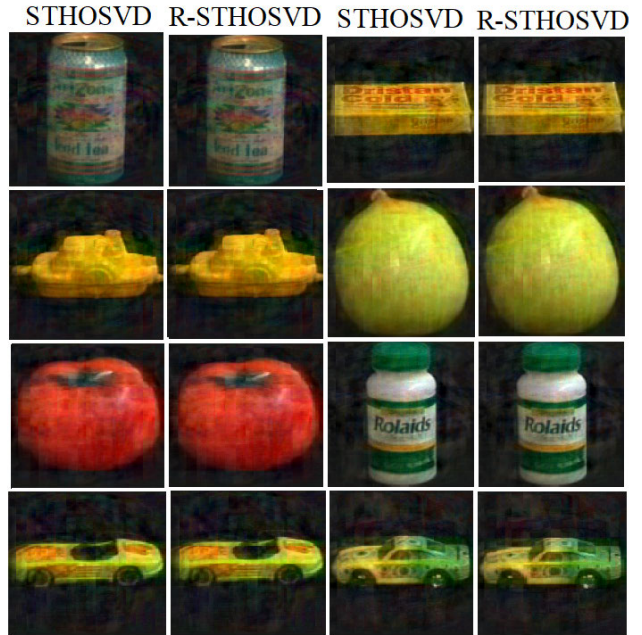
FIGURE 16. The reconstructed images using randomized and deterministic STHOSVD algorithms for the first 8 images.
