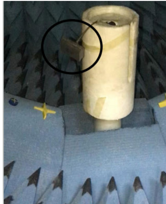
FIGURE 5. Measurement of the radiation pattern and gain in anechoic chamber.
