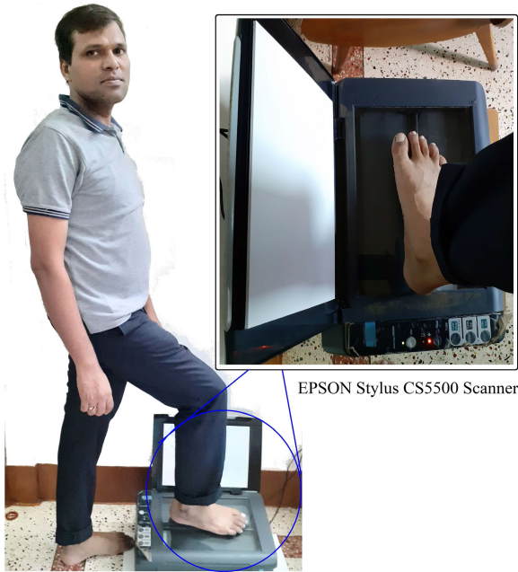
FIGURE 1. Experimental setup for footprint acquisition using EPSON Stylus CS5500 flatbed scanner.
