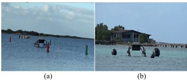
FIGURE 27. Our USV perform tasks in Unmanned Surface Vehicles Challenge in Hawaii. (a). USV detects and locates the post to complete the task; (b). USV autonomously passes through obstacle areas.
