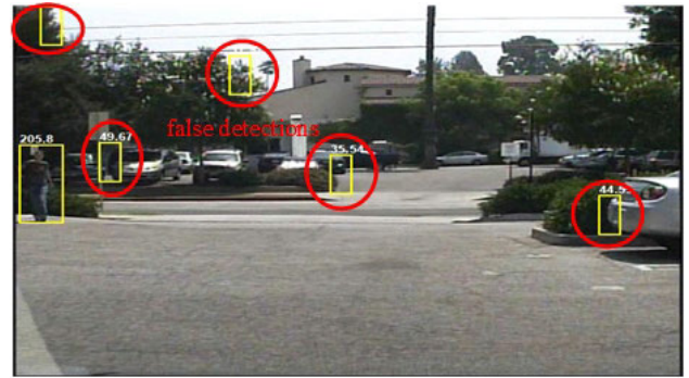
FIGURE 11. Illustration of false pedestrian detection.
