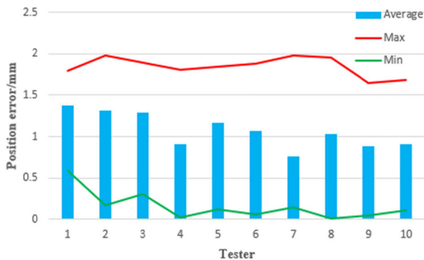
FIGURE 29. Guidewire position error.
