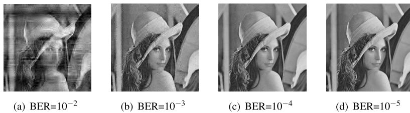
FIGURE 19. The recovered images of Wang's method when shadow images are added with different levels of Gaussian noise. 19(a) BER = 10^{-2} , PSNR=13.12 ; 19(b) BER = 10^{-3} , PSNR=22.67 ; 19(c) BER = 10^{-4} , PSNR=30.96 ;19(d) BER = 10^{-5} , PSNR=32.62 .
