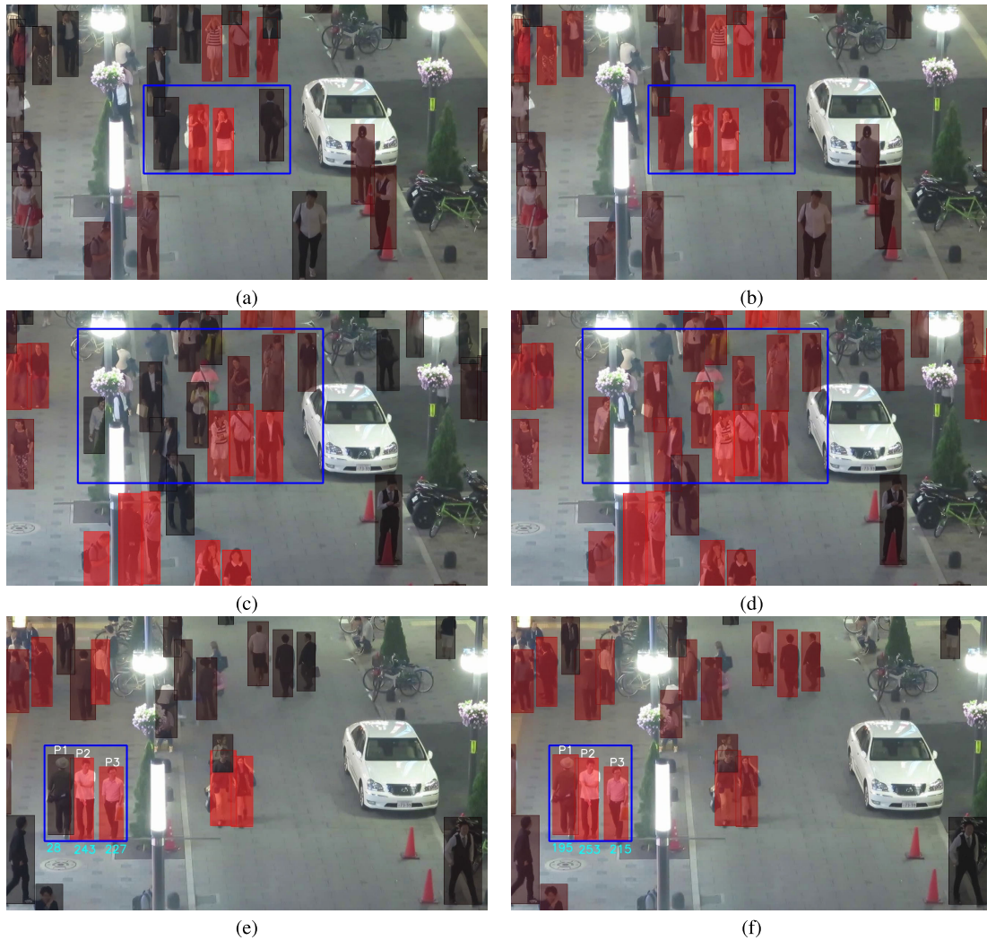
FIGURE 14. Application of proposed and density-based models to MOT16-03 (a-d) and MOT16-04 (e-f) videos, where the red color indicates a high score. The images in the left column (a, c, and e) represent the proposed results and those in the right column (b, d, and f) represent the density-based results. Note that the proposed method yielded high scores for persons in a group rather than for individual pedestrians, whereas the density-based method did not. Detailed comparisons for three pedestrians, shown in (e) and (f), are provided in Figure 15.
