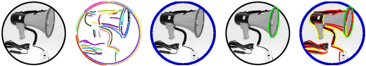
FIGURE 2. Geometry analysis obtained with the proposed method. From left to right: original image, contours detected using the method in [8], [9] (at a particular scale), detected circles (blue), ellipses (green) and joint detection including line segments (red), circular arcs (yellow) and elliptical arcs (orange). The initial contours at different scales are grouped into circles and ellipses, the rest are combined to form line segments, circular arcs or elliptical arcs. Curves that do not fall into any of these categories are not displayed in the final output. For simplicity only contours at a particular scale are displayed even if the procedure is multi-scale. See Fig. 5 for a more complete version of the figure.
