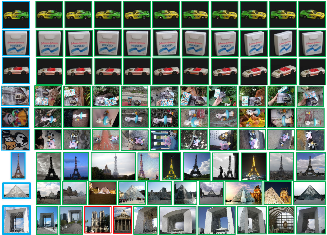
FIGURE 12. Top-10 retrieved images of COIL-100 (rows 1-3), INSTRE-M (rows 4-6) and Paris 6K (rows 7-9) datasets. The above results were obtained by using the colour neural descriptors that achieved best results in each dataset. The queries are framed with blue rectangles, correctly retrieved images with green ones and incorrectly retrieved images with red rectangles.
