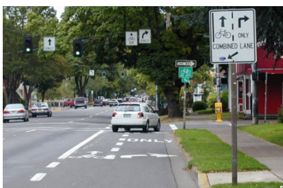
FIGURE 8. Combined bike lane/turn lane [7].
