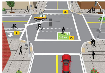
FIGURE 11. Two-stage turn queue boxes [138].
