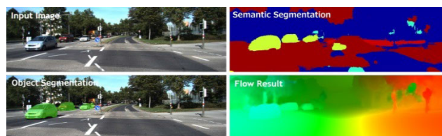
FIGURE 4. Optical flow estimation with semantic segmentation by using SOF model presented in reference [26].
