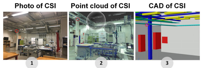
FIGURE 3. Step 1-3 From Scanning to CAD representation of the laboratory that serves as a test facility. The red circle marks the LTE Radio Dot installation position.
