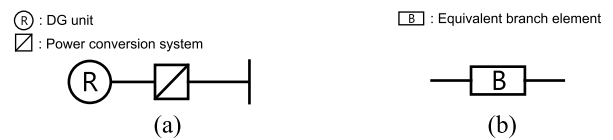
FIGURE 2. Single branch formation with series connection. (a) System diagram. (b) Block diagram of the equivalent model.
