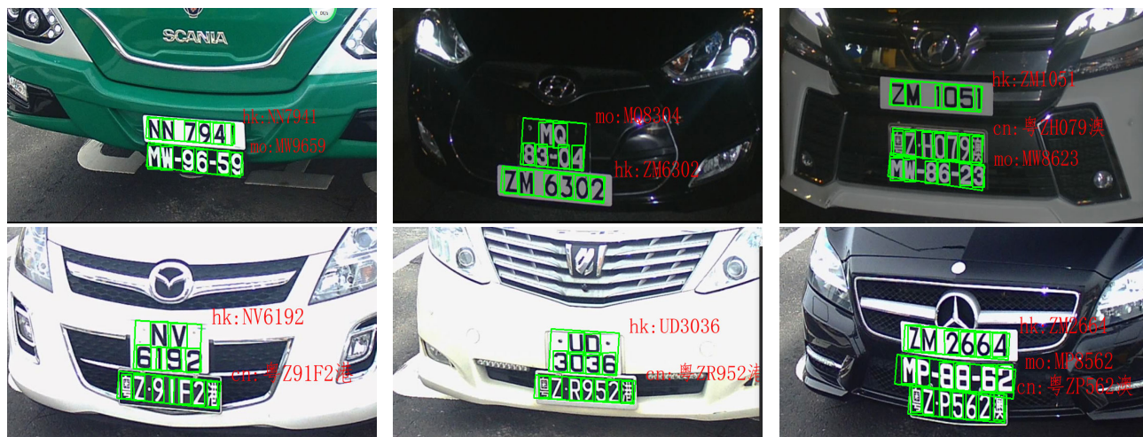
FIGURE 4. LPs have been detected and recognized, wherein “hk” means Hong Kong, “mo” means Macao, and “cn” means Mainland China.
