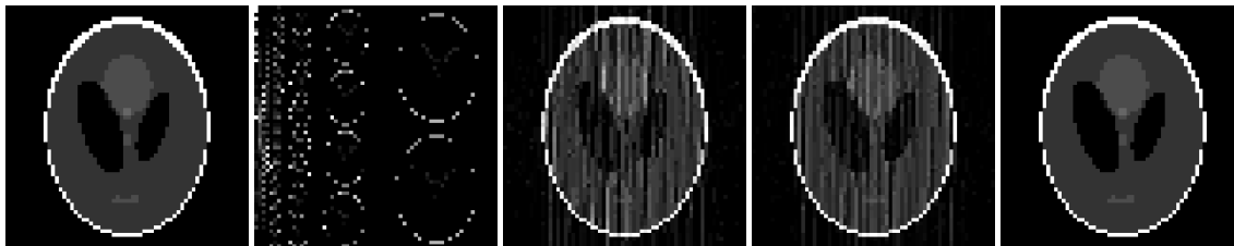
FIGURE 4. Reconstruction results. The first is the original image, the second is the sparse image after wavelet transform, the third is the image reconstructed by the OMP (PSNR=20.5912db, SSIM=0.6147), the fourth is the image reconstructed by the SVD-WOMP (PSNR=23.6668db, SSIM=0.6852), the last is the image reconstructed by the RE-WOMP with the weighting times n = 27 (PSNR=262.5134db, SSIM=1).
