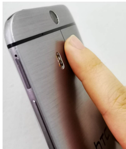
FIGURE 1. A video signal of the index fingertip which was obtained by using the rear camera of an HTC M8d smartphone.
