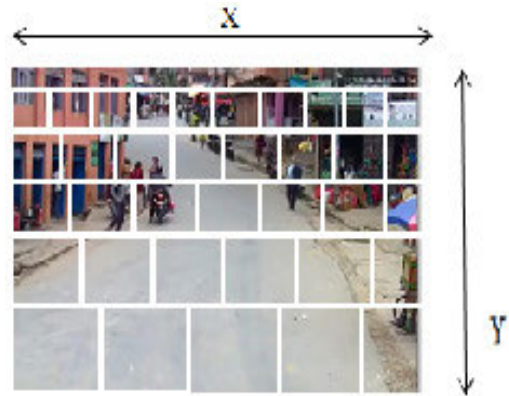
FIGURE 3. The cell structure of a scene. Different cell sizes are shown, where, regions closest to the camera are represented by larger cells, while regions away from the camera are represented by smaller cells.
