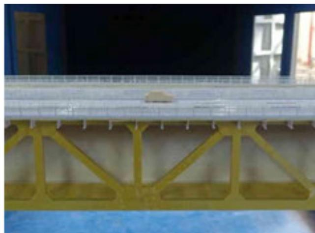
FIGURE 6. Wind tunnel test model.
