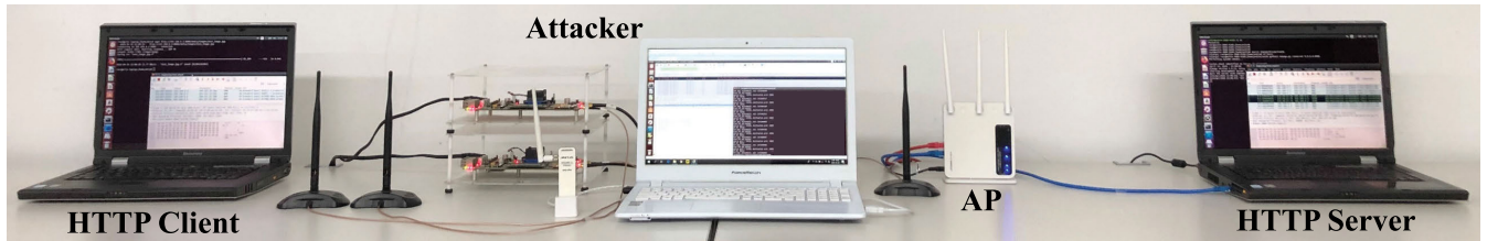
FIGURE 9. Malicious frame injection test-bed.
