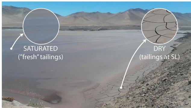
FIGURE 1. Thickened tailings deposit (TTD) in drying process.
