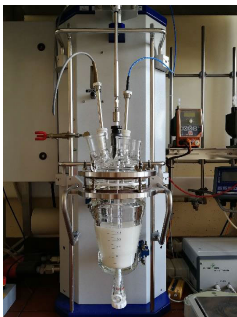
FIGURE 25. Laboratory batch bioreactor used for tests, analyses, and control implementation.
