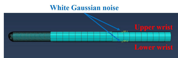
FIGURE 7. Sideview of 3D finite element hand model.
