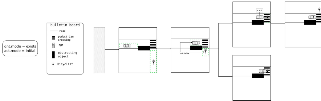
FIGURE 15. A Traffic Sequence Chart for an abstract scenario in which an object occludes a bicyclist at a pedestrian crossing.
