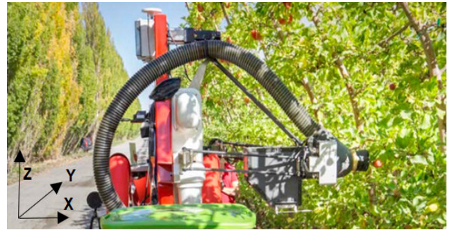
FIGURE 1. Vacuum-tube type gripper that transports the harvested fruit to a bin via the vacuum tube (abundant robotics harvester; photo courtesy of TJ mullinax/good fruit grower).
