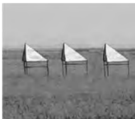
FIGURE 2. The array of corner reflector on the ground [3].
