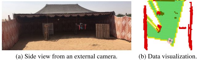
FIGURE 16. Experimental verification of the indoor motion planning and exploration techniques in the desert near Abu Dhabi, United Arab Emirates before MBZIRC 2020. In the image on the right, the red blocks denote obstacles, the green blocks show the already scanned space, and the yellow blocks denote frontiers for exploration. A video from this experiment is on YouTube 12 .
