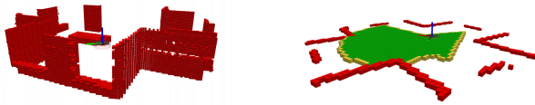
(a) A visualization of an occupancy grid stored in a three-dimensional buffer. The size of the grid is 128 \times 128 \times 32 with resolution of 0.1 m.
