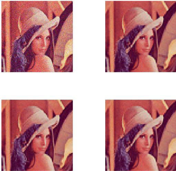
FIGURE 5. The blurred image (top left), the restored image by Algorithm 1 (top right) (SNR = 16.77, PSNR = 22.11, SSIM = 0.9138), by Algorithm 2 (bottom left) (SNR = 16.74, PSNR = 22.07, SSIM = 0.9131) and by Algorithm 3 (bottom right) (SNR = 16.77, PSNR = 22.10, SSIM = 0.9137).
