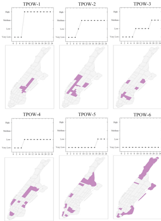
FIGURE 12. Six unique temporal patterns of non-checkerboard co-clusters for weekdays. The y-axis represents the travel states.
