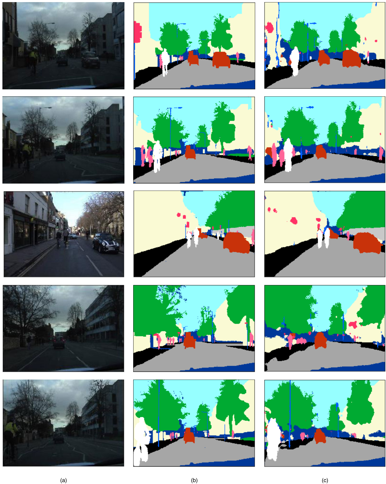
FIGURE 8. (a) Input image, (b) target annotated image from the CamVid database, and (c) generated segmented image using the proposed model.
