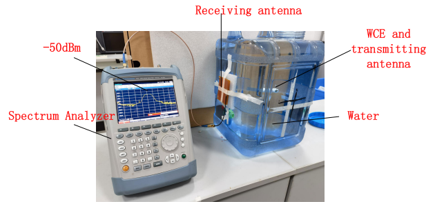
FIGURE 12. The received power is compared when flexible monopole antenna and dielectric resonance antenna as transmitting antenna, respectively.
