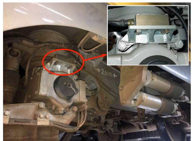
FIGURE 5. Accelerometer and its installation on axle box.
