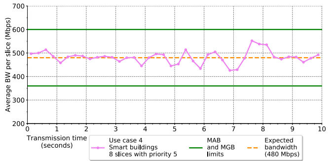
(d) Use case 4: Video surveillance in Smart Buildings 8 Smart buildings, each one equipped with 100 IP video cameras, transmitting a total of 320,000 PPS Total BW achieved: 3.848 Gbps.
