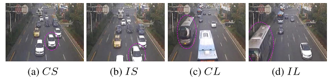
FIGURE 3. Interpretation of vehicle classification. (a) Complete small vehicle ( CS ). (b) Incomplete small vehicle ( IS ). (c) Complete large vehicle ( CL ). (d) Incomplete large vehicle ( IL ).
