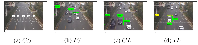
FIGURE 7. Interpretations of the lane, the illustration of calculating process of k and b , and an example. (a) The four lanes. (b) The vehicles in the distance. (c) The vehicles in the near. (d) The example.
