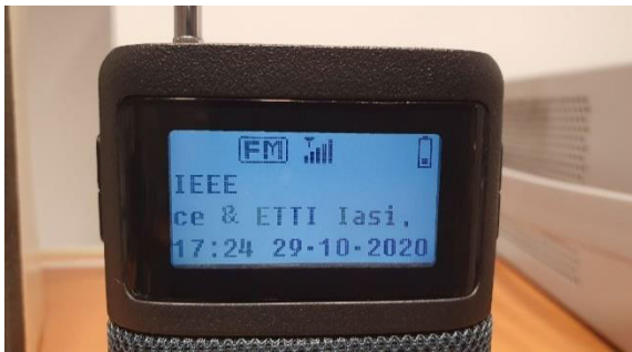
FIGURE 32. RDS message decoded by a commercial FM radio receiver.
