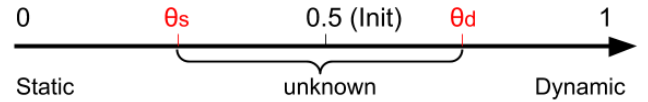
FIGURE 11. Moving probability. \theta_s is the static threshold and \theta_d is the dynamic threshold value.
