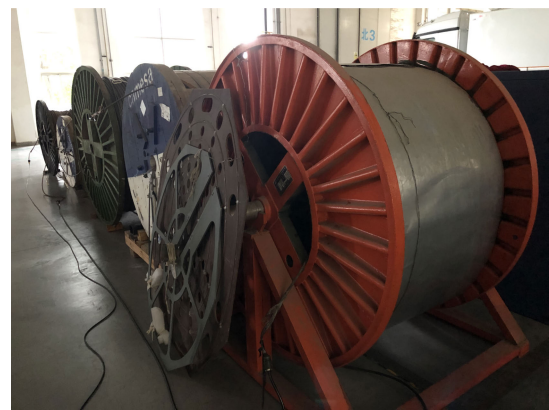
FIGURE 23. 7km armored cable.
