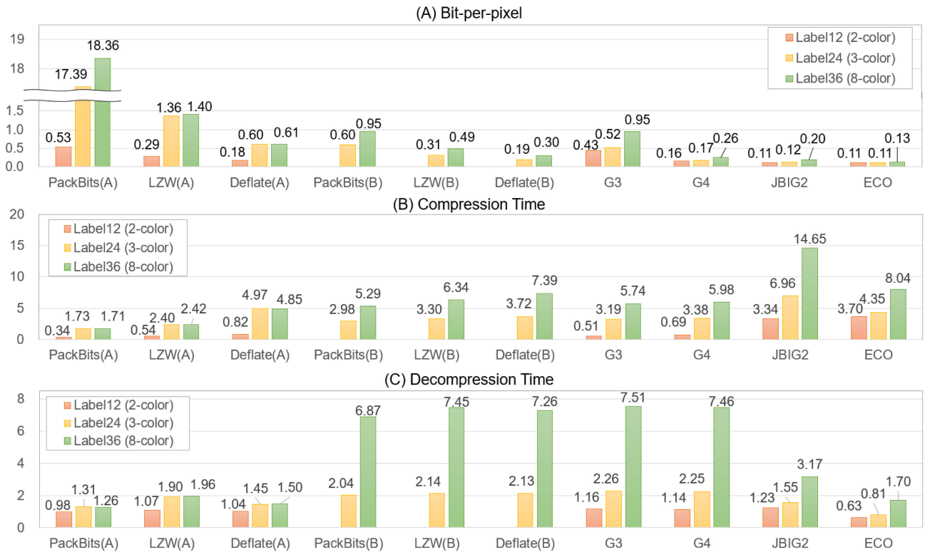
FIGURE 19. Performance results of the algorithms for the images with Label12, 24, and 36.
