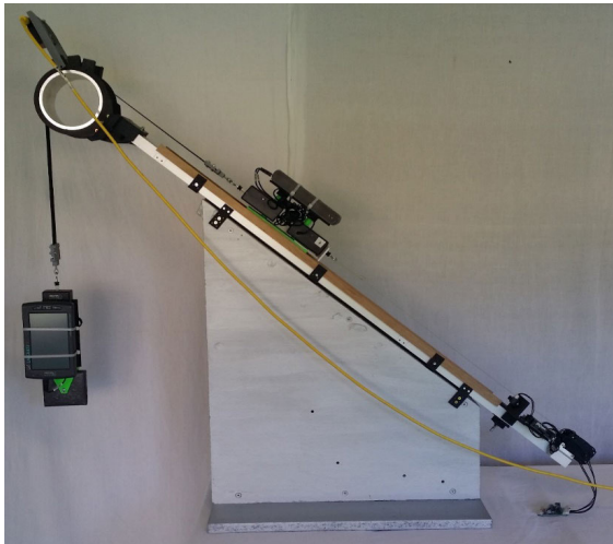
FIGURE 6. Side view of the measuring assembly with the cylindrical surface set at an angle of wrap 45°.
