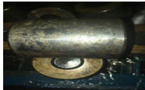
b. Wind turbine gearbox bearing rolling element pitting
