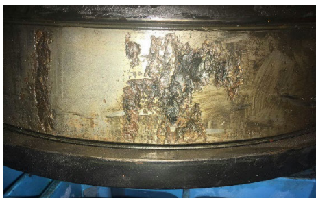
a. Wind power gearbox bearing inner ring peeling off
